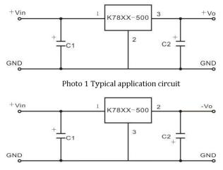
Photo 2 Negative output application circuit
